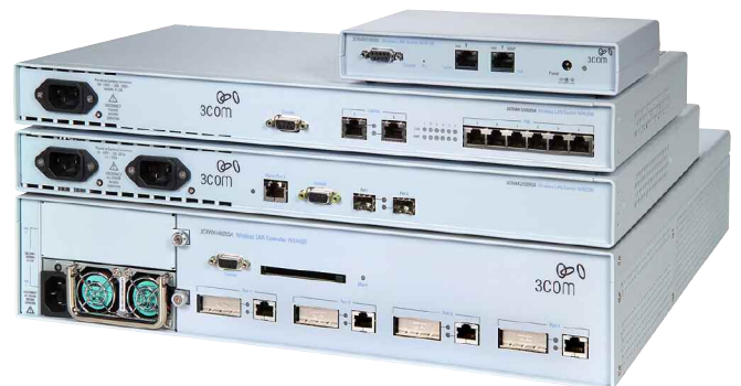
from top: 3Com WXR100 Remote Office Wireless LAN Switch, Wireless LAN Switch WX1200, Wireless LAN Controllers WX2200 and WX4400
